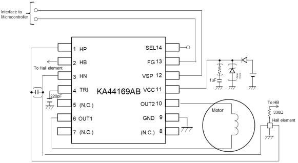
Note: The recommended circuit is an example. The operation of the mass production set is not guaranteed. Sufficient evaluation and verification is required in the design of the mass production set. Customer is fully responsible for the incorporation of the above illustrated application circuit in the production.
